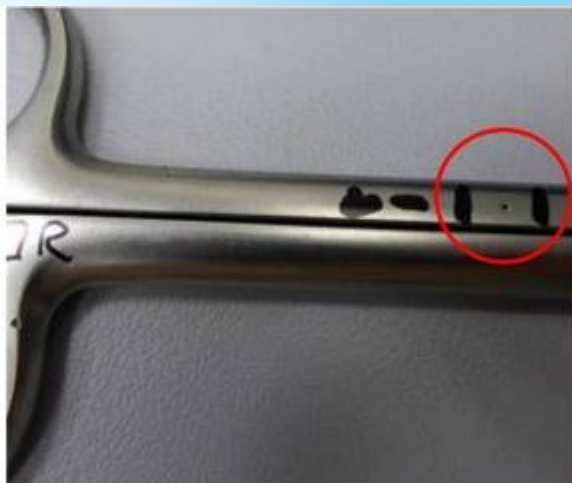
Example: Old Pitting Corrosion here 63µg Protein
