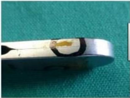
Instruments picked from working Sets primary Assessment: Corrosion
